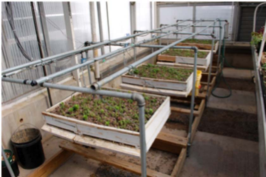
Figure 5. Plant growth in roof assembly boxes 4 weeks after planting cuttings.
