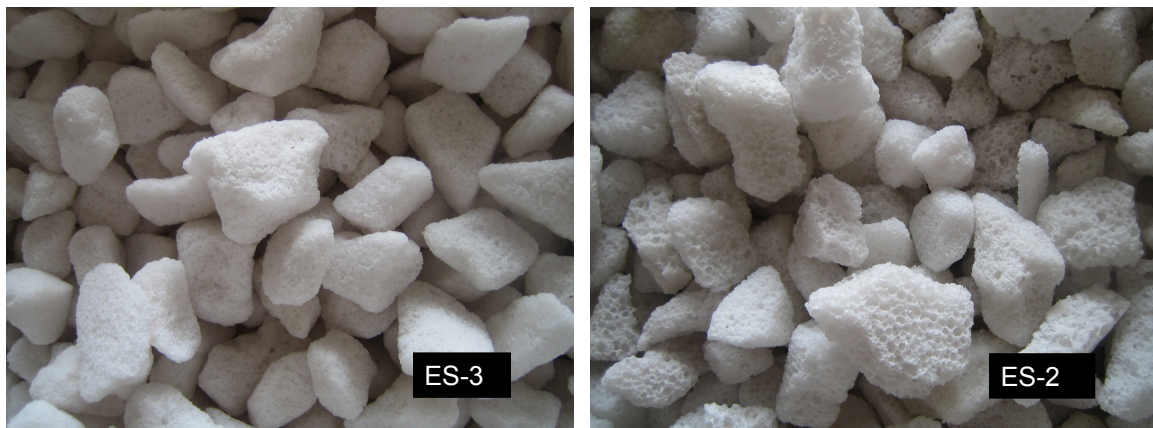
Figure 1. Two different formulations of Earthstone crushed foamed glass. Left, ES-3 characterized by small pore size for increased water retention and perfectly balanced water to air ratio with 45% water and 45% air at saturation (v/v, %). Right, ES-2 characterized by larger pore size with 40% water and 52% air at saturation (v/v, %) for increased drainage.
